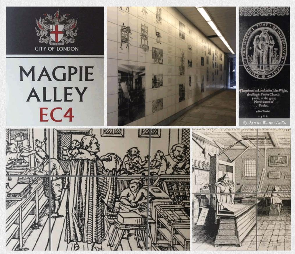
A printing office (1600). The printing press is at the back left, with a printer about to pull the handle which lowers the top plate of the press on to the paper, which is resting on top of the freshly-inked type, The compositor's trays are seen on the right. Compositors (1606):. Note the trays with compartments for the individual letters at the back
